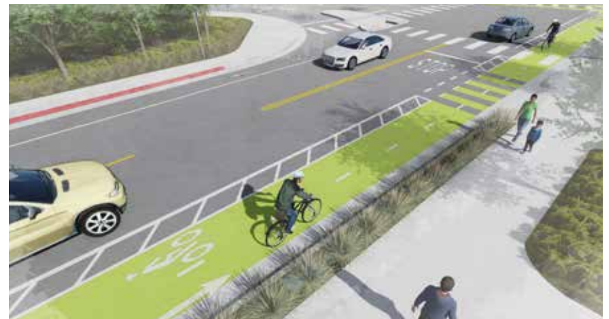
Example of a Class II bike lane with painted lanes and buffer
