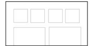
Opening sizes have been increased to better relate to mass of building.
