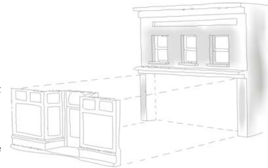
Storefront remodel should (where possible) re-create the historic architectural character of the storefront.
