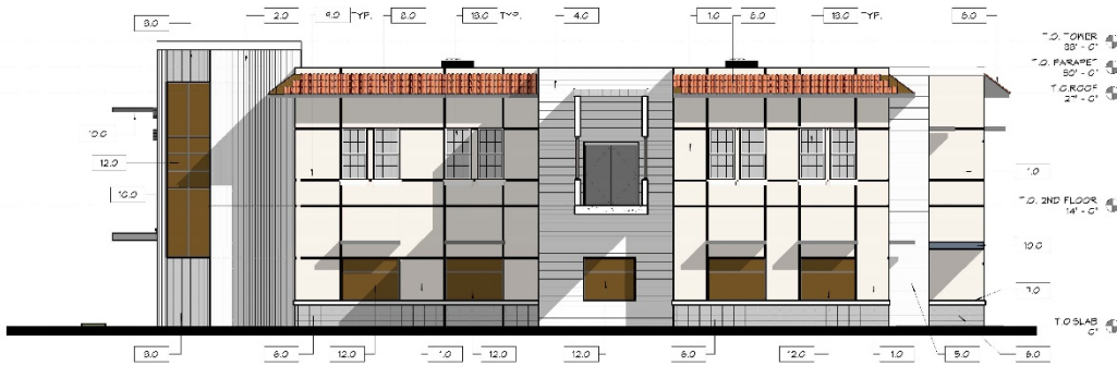
1 EXTERIOR ELEVATION - NORTH 1/8" = 1'-0"
