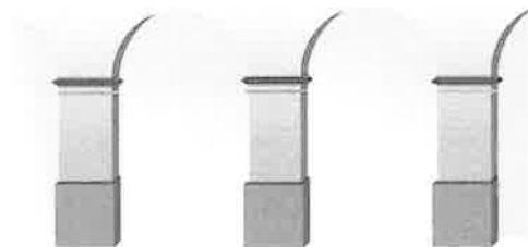
A "blind" arcade is an example of a simple design element that adds depth to an otherwise flat expanse of wall.
